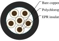
Bare copper conductor Polychloroprene rubber outer jacket EPR insulation
